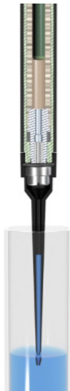
Figure 3–1: Air displacement pipetting principle
