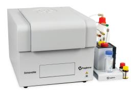
The Innovate<sup>™</sup> System performs high-throughput screening of products. It rapidly detects adenosine triphosphate (ATP), the energy-releasing molecule found in every living cell. To ensure only microbial ATP is counted, an enzyme breaks down the cell, which isolates microbial ATP.
