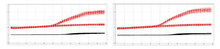
Figure 2: BAX System PCR Assay for Salmonella (KIT2011) Capped (Left) and Uncapped (Right) Lysates
