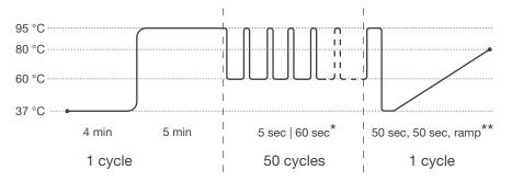
Pre-incubation: 1 cycle Step 1: 37 °C for 4 min Step 2: 95 °C for 5 min
