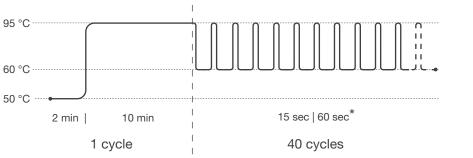
Pre-incubation: 1 cycle Step 1: 50 °C for 2 min Step 2: 95 °C for 10 min Amplification: 40 cycles Step 1 : 95 °C for 15 sec Step 2\*: 60 °C for 60 sec
