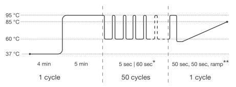
Pre-incubation: 1 cycle Step 1: 37 °C for 4 min Step 2: 95 °C for 5 min
