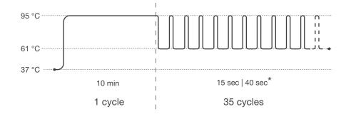
Pre-incubation: 1 cycle Step 1: 95 °C for 10 min Amplification: 35 cycles Step 1: 95 °C for 15 sec Step 2\*: 61 °C for 40 sec
