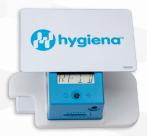
Test configurations are uploaded via RFID before the measurement. Put the lot specific RFID card onto the top side of the device or hold the device against the RFID tag sticking on the test box until the configuration data has been uploaded (audible signal).
