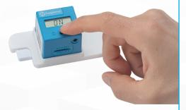
To turn on the device press the button briefly, less than 1 second.
