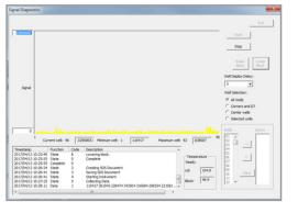
5. If the signal appears relatively low and uniform across the wells, the sample block does not need to be cleaned at this time.
