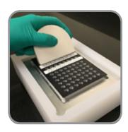
Tilt the tool backward so that the caps lift off.
