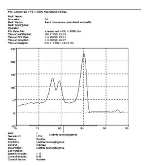
**Individual Well Report:** Provides a detailed report for each sample selected (up to 96 samples), including the melt curve image as displayed in the Well Detail View.
