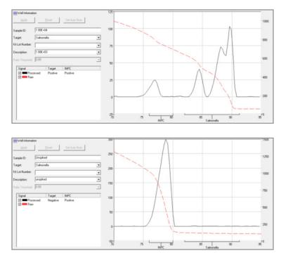
Typical positive (top) and negative (bottom) melting curve profiles
