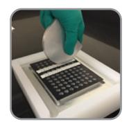
Roll the tool over the strip to lock the caps in place.
