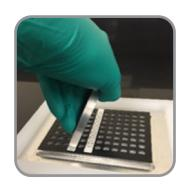
Tilt the tool forward and push down so that it locks over the caps.
