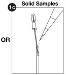
1c. Solid Samples: Add 1 mL of 10% w/v suspension of solid sample directly to RT Enrichment Device.
