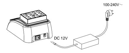
1.3.3 To power ON the incubator, turn the power switch to "I". The incubator is ready to operate when the display becomes visible.
