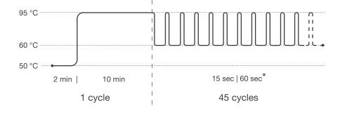
Pre-incubation: 1 cycle Step 1: 50 °C for 2 min Step 2: 95 °C for 10 min Amplification: 45 cycles Step 1: 95 °C for 15 sec Step 2\*: 60 °C for 60 sec
