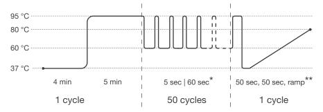
Step 1: 37 °C for 4 min Step 2: 95 °C for 5 min Amplification: 50 cycles Step 1: 95 °C for 5 sec Step 2\*: 60 °C for 60 sec Melting Curve: 1 cycle Step 1: 95 °C for 50 sec Step 2: 37 °C for 50 sec
