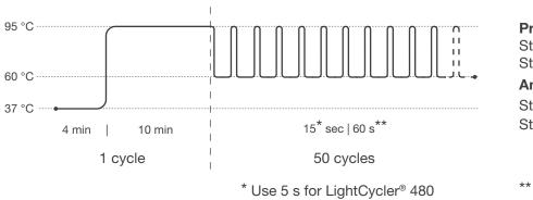
Pre-incubation: 1 cycle Step 1: 37 °C for 4 min Step 2: 95 °C for 10 min Amplification: 50 cycles
