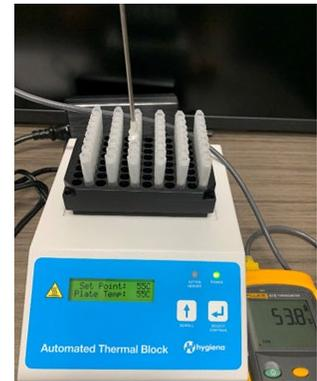
Press the SCROLL button to increase the value of the set point to 95 °C. The block automatically begins the heating process.
