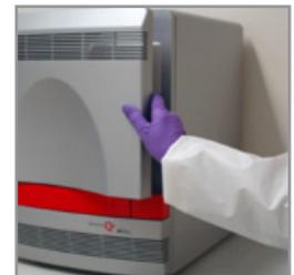
4. Pull the lamp release lever forward to release the halogen bulb from its mount.
