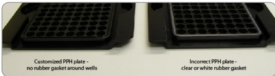
1. **The customized PPH plate does not have a rubber gasket around the perimeter of the wells.** The incorrect PPH plate may have a clear or white-tinted rubber gasket around the wells.
