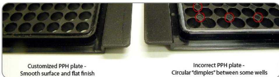
3. **The surface of the customized PPH plate is smooth and has a flat (not shiny) finish.** The incorrect PPH plate has a shinier finish and has circular "dimples" between some of the wells.
