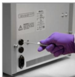
3. Remove each fuse from its holder and inspect for damage. Carbon typically coats the inside of failed fuses.
