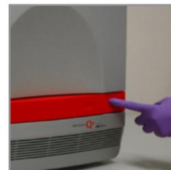
If you need to shut down the system for seven or fewer days, simply check that no rack is in the tray, then press the power button to power down the BAX® System instrument.
