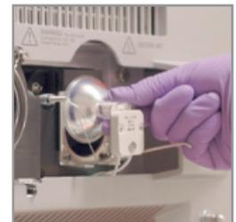
6. Push the lamp release lever back into the upright position.
