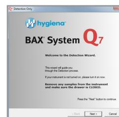
3. A new screen automatically appears as the instrument heats to its set temperatures. The red color in the banner indicates that it is a Detection Only run.
