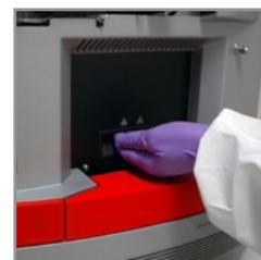
3. If the error light continues to display, check the monitor. If you don't see the desktop for the Windows operating system, turn off power to the instrument and wait for the monitor to display the desktop. Then power on the instrument.
