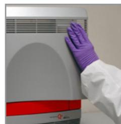
2. If the error light continues to display, open the instrument door and pull on the heated cover to verify that it is fully forward. Close the instrument door.
