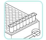
Note: Time and g-force depend on the centrifuge (please see 2.1. Required Material for more information). Set the centrifuge acceleration to maximum speed and the brake to medium. If necessary, centrifugation forces should be calculated according to the manual of the used centrifuge.
