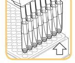
Take care that the tips of the pipette in the reaction tubes are not touching the pellets.
