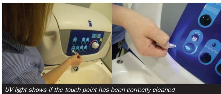
UV light shows if the touch point has been correctly cleaned
