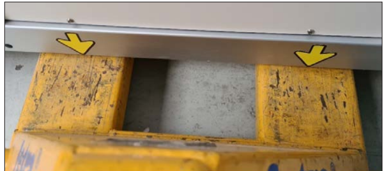
Fork placement when lifting the Autosampler III
