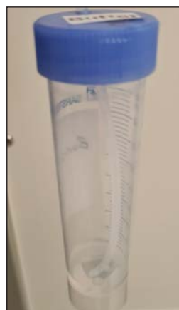
Correct position of tubing inside the tube
