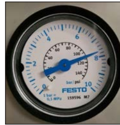
Sufficient pressure >5 bar
