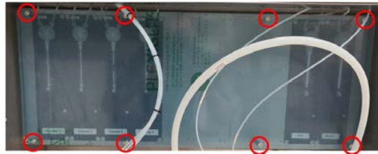
Picture of cover plate and screw points
