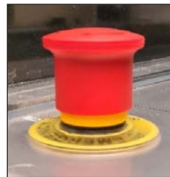
"Emergency" button unpressed (to reset turn counterclockwise)
