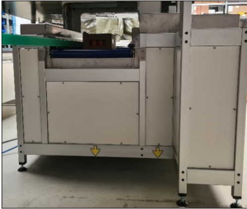
Lifting points, left side Autosampler III
