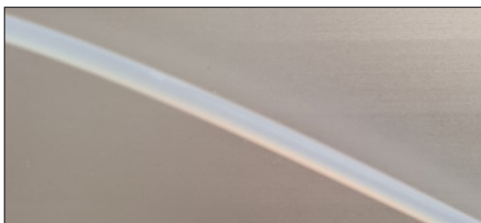
Correct tubing (little to no air bubbles)
