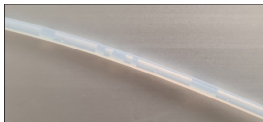
Incorrect tubing (significant amount of air)
