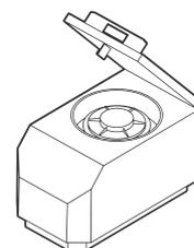
**Centrifuge** suitable for 5 - 50 mL tubes and capable of a 3,500 × g centrifugal force
